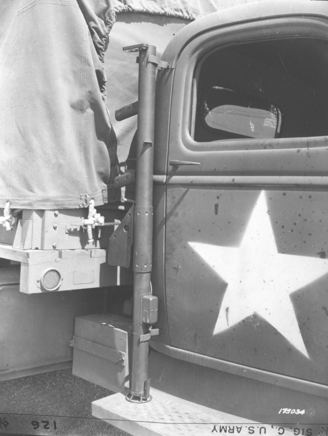
Rocket gun mounted on a 1/2 ton vehicle. Camp Gruber, Okla. 4/3/43; 788th Ordnance (111-SC-175034)
